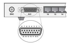
Fig. A-3 AUI Connector on Rear Panel
